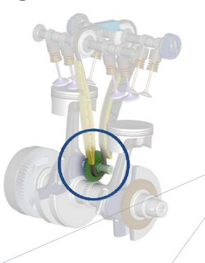
Centre cam drive with idler gear for smaller camchain sprockets
